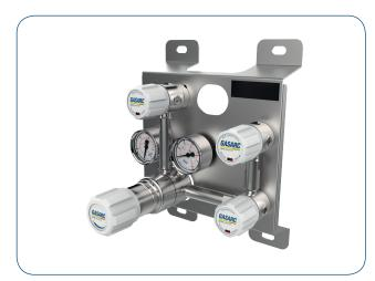
The Spec Master HPM6210 Series single stage single cylinder manual change control panels are designed for primary pressure gas control of non-corrosive or toxic, high purity gases up to grade 6.0 purity (99.9999%), on gas distribution systems where slight pressure variation is acceptable.
